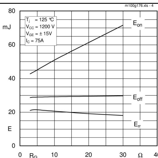
Fig. 4 Typ. turn-on /-off energy =  $f(R_G)$
