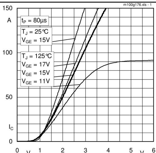
Fig. 1 Typ. output characteristic, inclusive  $R_{CC} + EE'$
