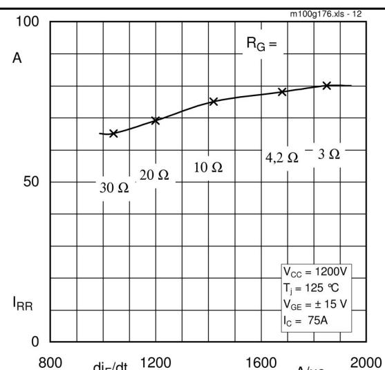
Fig. 11 Typ. CAL diode peak reverse recovery current
