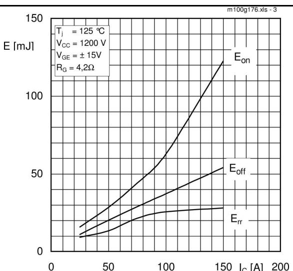
Fig. 3 Typ. turn-on /-off energy =  $f(I_C)$
